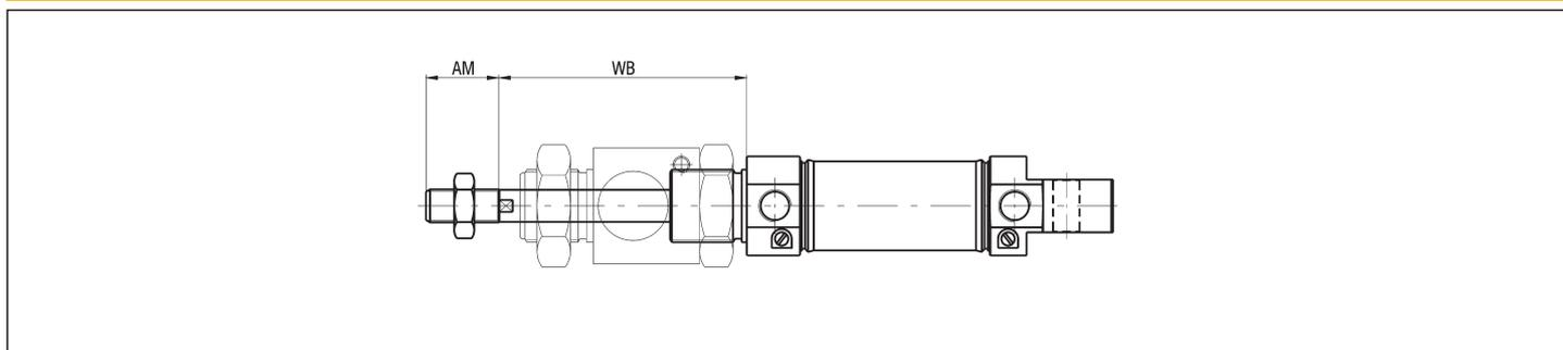
P.S.: End cap nut and rod nut supplied as standard
