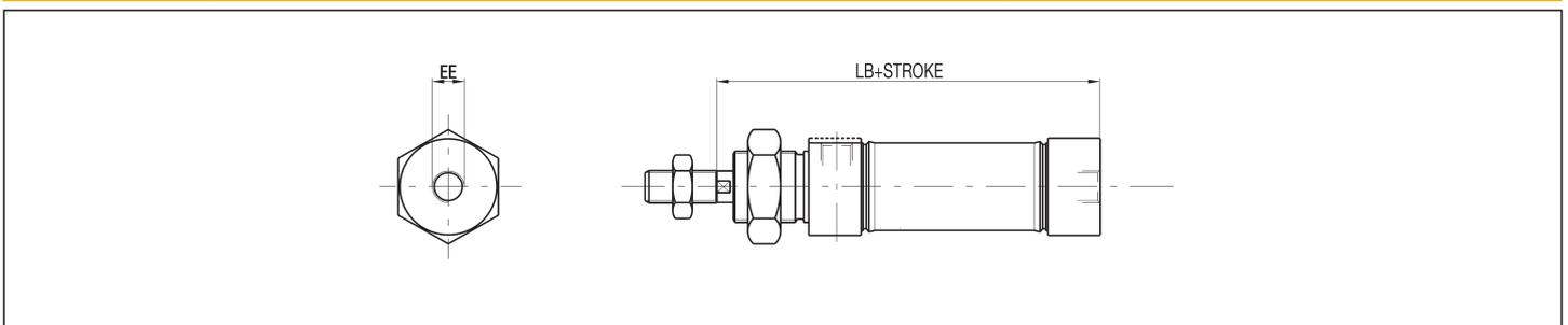
P.S.: End cap nut and rod nut supplied as standard
